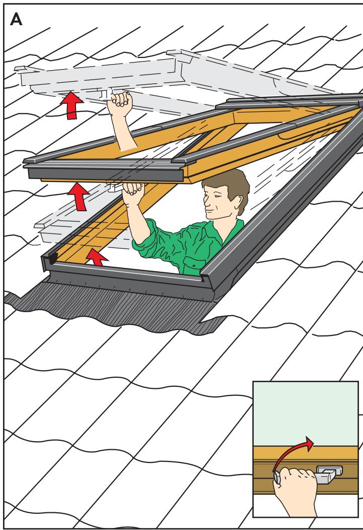
**ENGLISH:** Open window by turning handle to vertical position. The sash should be able to remain open in any position. If not, check that fittings and springs connect on both sides (see section **B**). If the sash still cannot remain open in any position, adjust springs (see section **C**).
