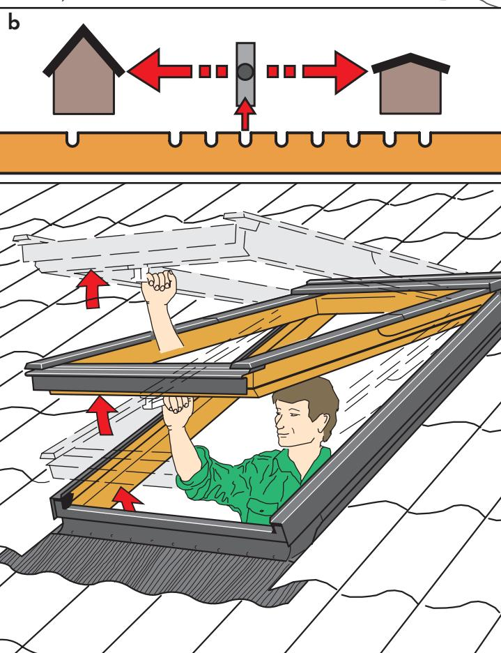
**ENGLISH: Connecting springs to fittings:** Close window using control bar (**a, b**). Then open window using handle on bottom of sash (**c**). Push sash outwards, ensuring that fittings and springs on both sides automatically connect (**d**).
